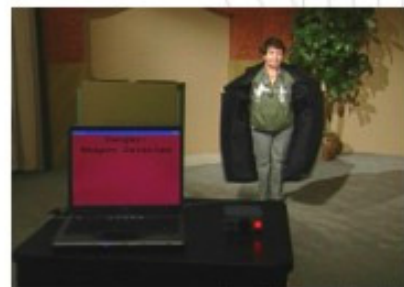
System scans and decides this individual is NOT safe (note bomb jacket underneath coat)
